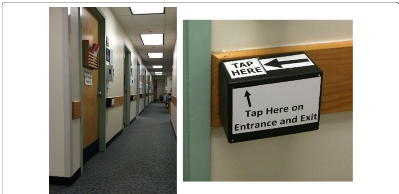
Fig. 5 RFID system in the clinic: custom-made RFID receivers were installed outside of clinic exam rooms with reminder signs instructing patients to swipe before and after entrance
